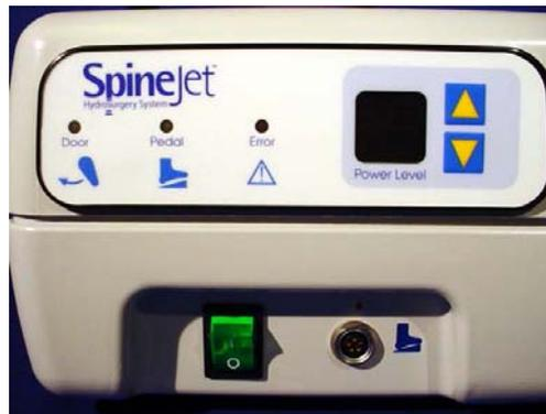
The Power Switch is on the lower left corner of the front panel. When the system is not in use, this switch should be in the off (0) position.
