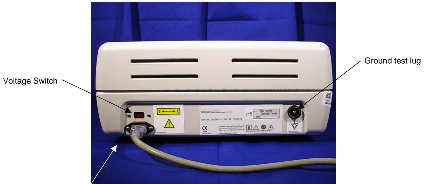
The Power Cord Receptacle and Power Cord utilized for connection to the electrical supply.
